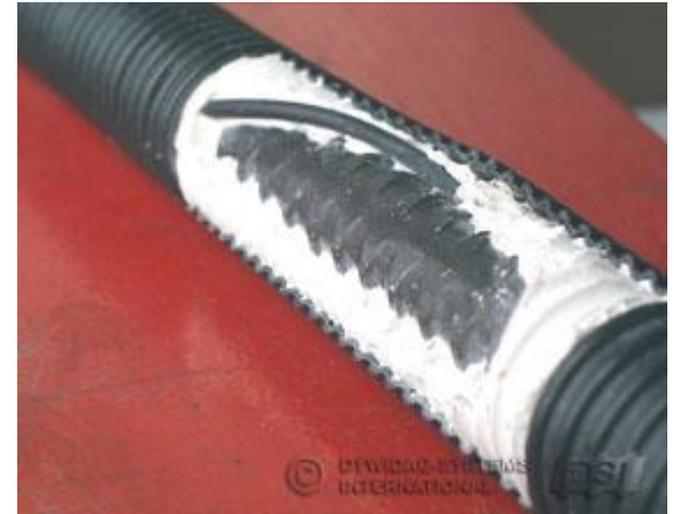
Strain gauge attached
