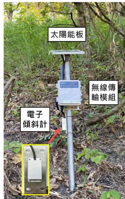
邊坡滑動監測桿
