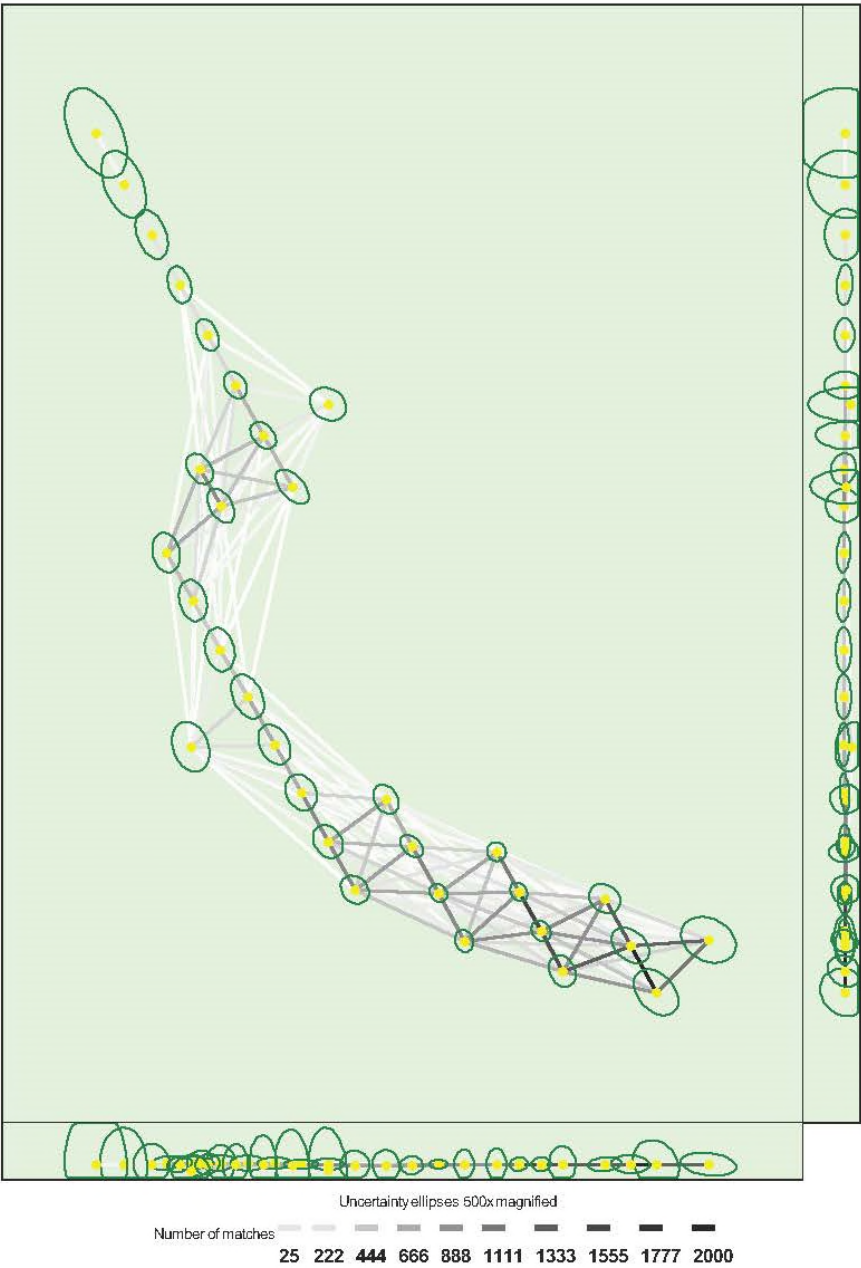
Figure 5: Computed image positions with links between matched images. The darkness of the links indicates the number of matched 2D keypoints between the images. Bright links indicate weak links and require manual tie points or more images. Dark green ellipses indicate the relative camera position uncertainty of the bundle block adjustment result.
