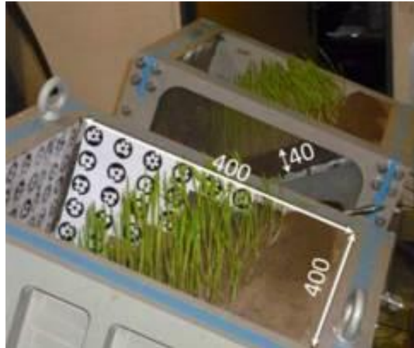
圖 2-12 燕麥於離心模型試驗中之生長情形 (Askarinejad, A. and Springman, S.M., 2015)
